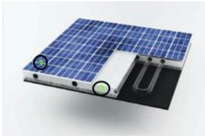
Figure 2.7: PV panel with phase-change materials [22]
