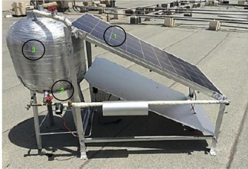
Figure 2.6: Hybrid photovoltaic/thermal (PV/T) system cooled by forced water circulation [20].
