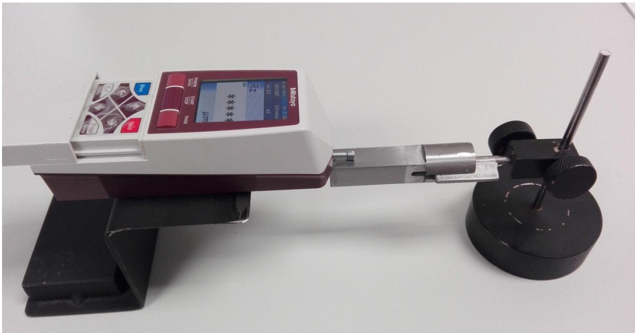
Figure 3.6: The clamping of the mould and surface roughness measurement setup.
