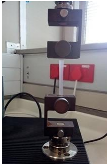
Figure 3.10: PCU film sample mounted on nominal gauge and two steel grips.
