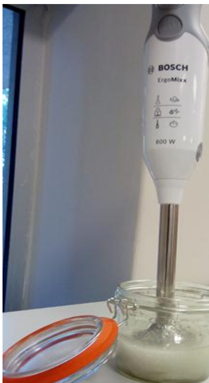
Figure 3.4: Bosch MSM66110 hand blender used in mixing the PC3595A-clear with N, N-dimethylacetamide solvent.
