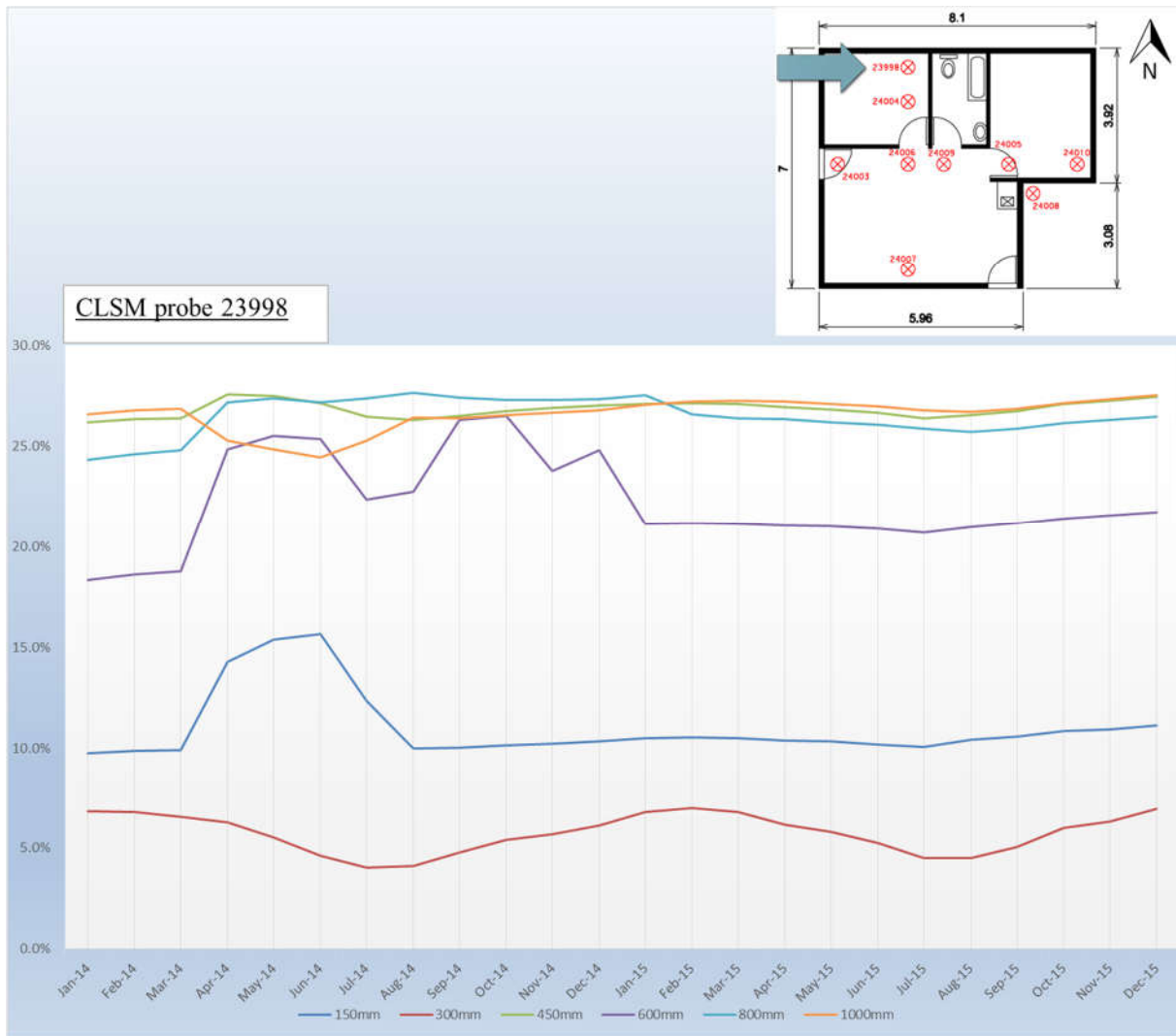
Figure 4-13: CLSM probe 23998 monthly average moisture variation for 2014 and 2015
