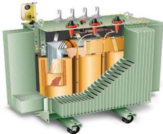
Figure 1: Power transformer construction [2]
