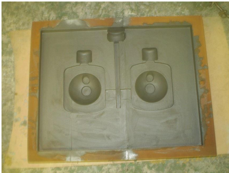
Figure 4: Drag component of the mould with the internal cavity of the tool to be cast.
