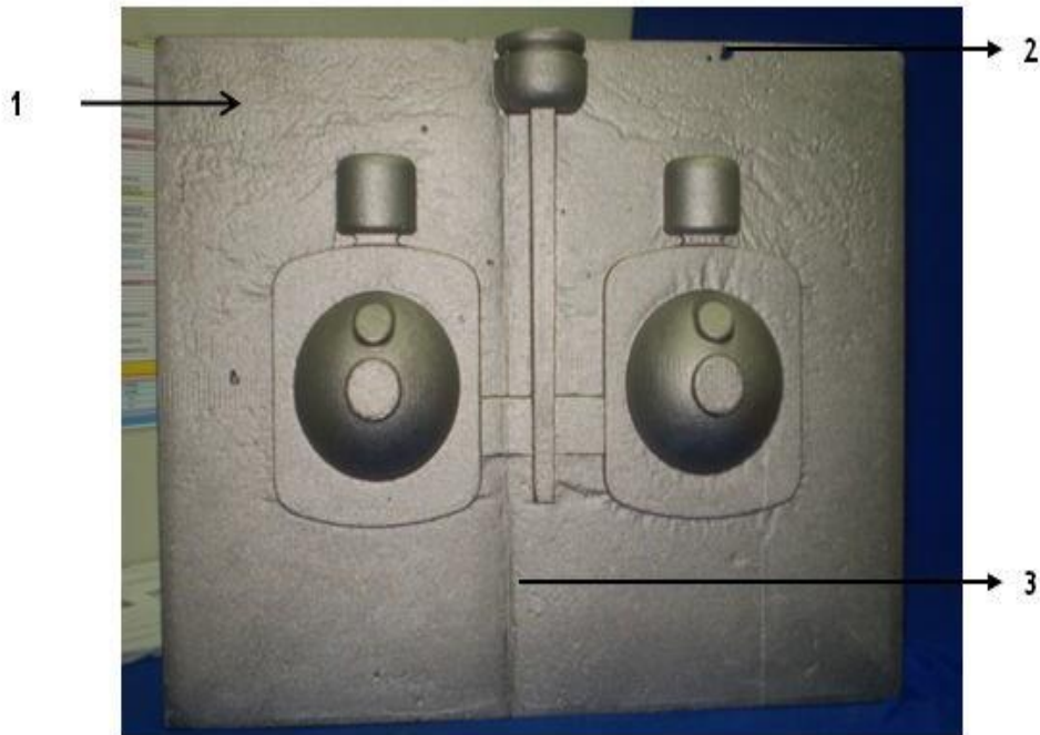
Figure 6: Final casting exhibiting some defects: 1: cold lap; 2: porosity; 3: Alignment fault
