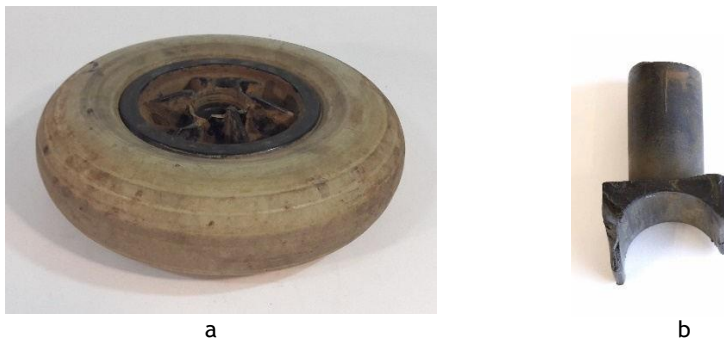
Figure 1 Front caster wheel (a) and seat post guide (b).
