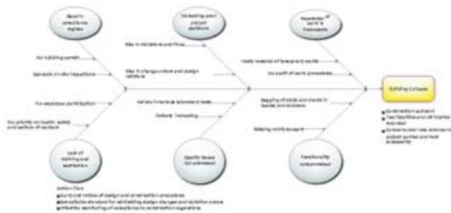
Figure 7: Additional causal factors of the collapsed building
