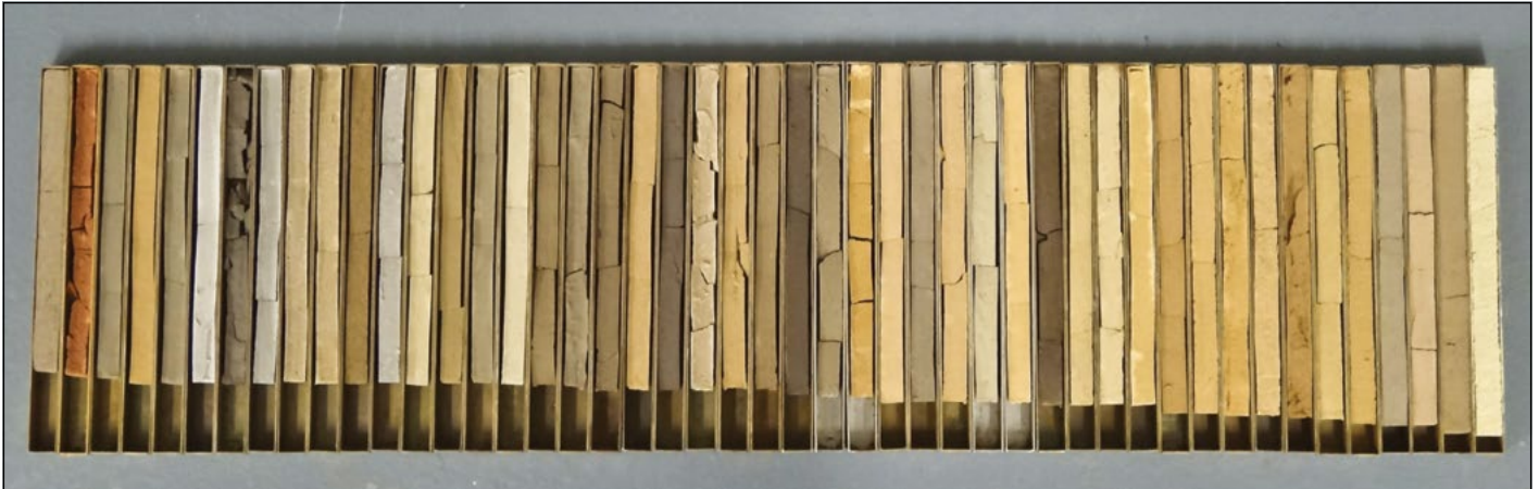
Photo 4 Shrinkage troughs: air-dried samples of some of the soils used in this investigation – the range of linear shrinkage shown here is from less than 5% to just over 20%; the red clay second from left is a raw (un-sieved, undried) sample from Gauteng which received no preparation other than mixing with de-ionised water (raw PI = 42); the samples on either side of it were extracted by wet preparation from two Free State soils and were not added back to the dry-sieved fines (PI = 49 and PI = 46); raw samples typically show more fracturing than fines-only samples; linear shrinkage of air-dried samples corresponded well with several heave indicators not dealt with in the TMH1 and SANS 3001 procedures
