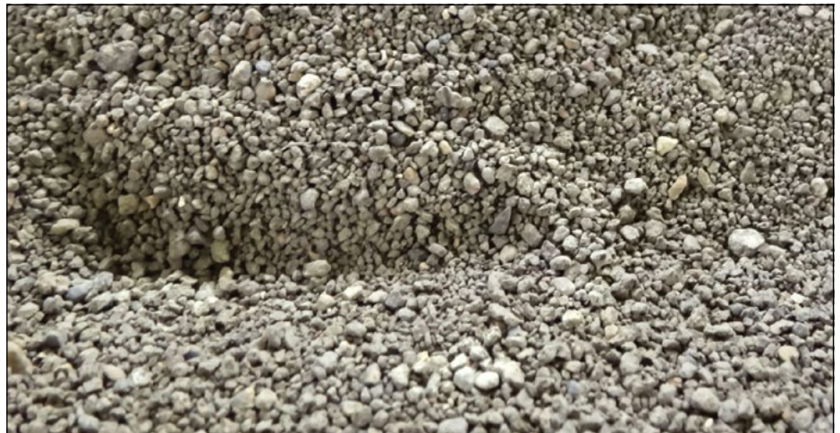
Photo 5 Material retained on the .425 sieve after prolonged grinding in the mortar; despite appearing to be hard gravel, more than 80% of this material passed the .425 sieve with wet preparation
