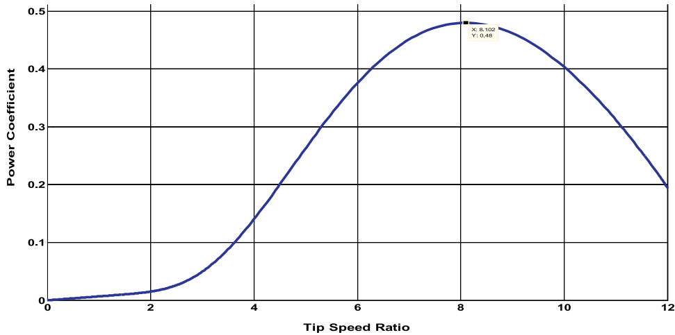
Fig. 2. Power coefficient versus tip-speed ratio of the turbine (with \beta = 0^\circ ).
