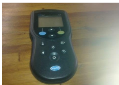
Figure 4.1 Hach HQd hand-held meter
