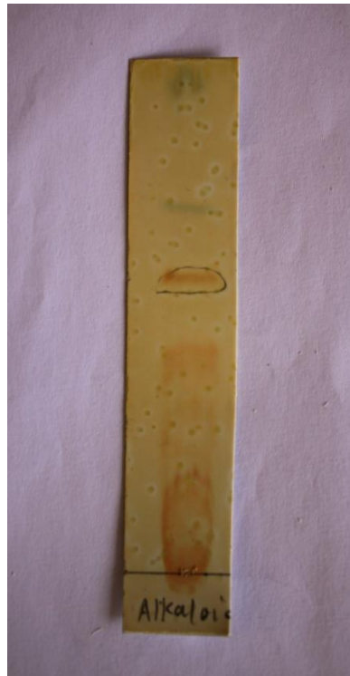
Figure 2.2: A chromatogram developed with Toluene/Chloroform/Ethanol (5.7:11.4:2.9) indicates the presence of alkaloids in the extracts of Buxus macowanii . An orange colour indicates the presence of alkaloids.
