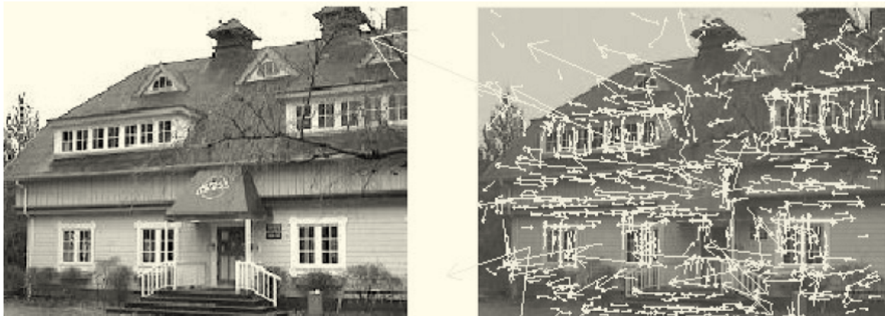
Figure 2-8: Image matching using Scale Invariant Feature Transform (SIFT) (David Lowe, 2004)
