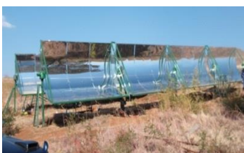
Figure 2.2 Photo of the parabolic trough collectors
