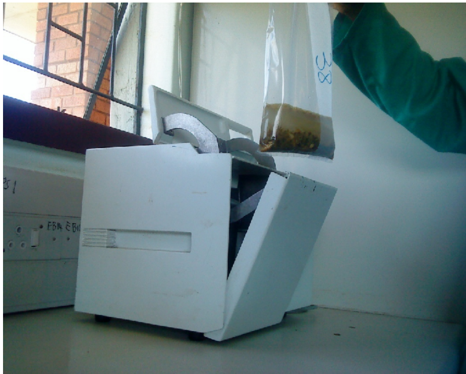
Figure 3.2: A 40 g silage sample in a stomacher
