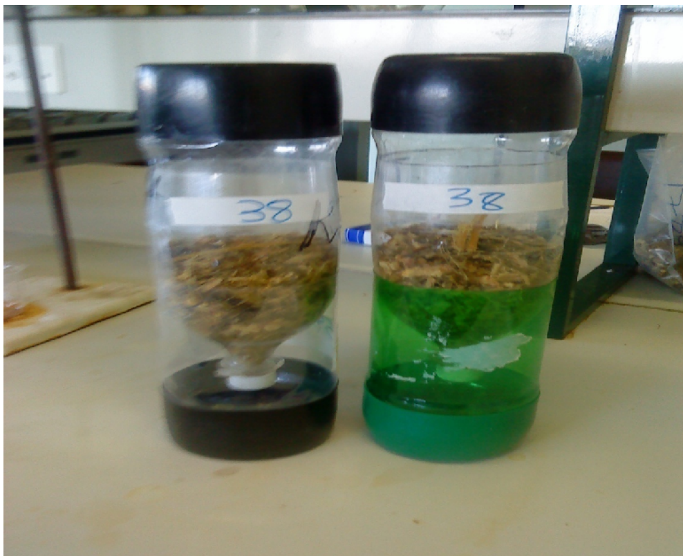
Figure 3.3: Aerobic stability test in 2-litre polyethylene terephthalate bottles
