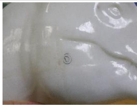
Figure 20 Air bubble entrapped
