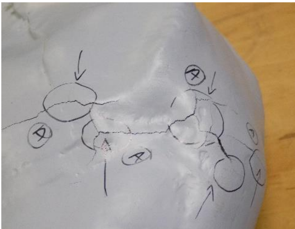
Figure 13 Cracks on surface of specimen 1
