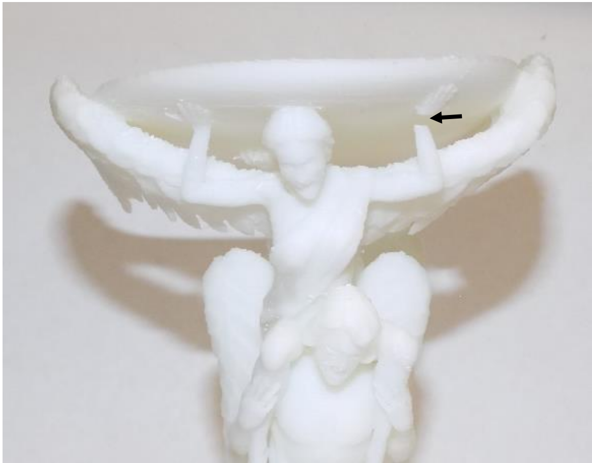
Figure 5 Angel arm broken during Post-processing
