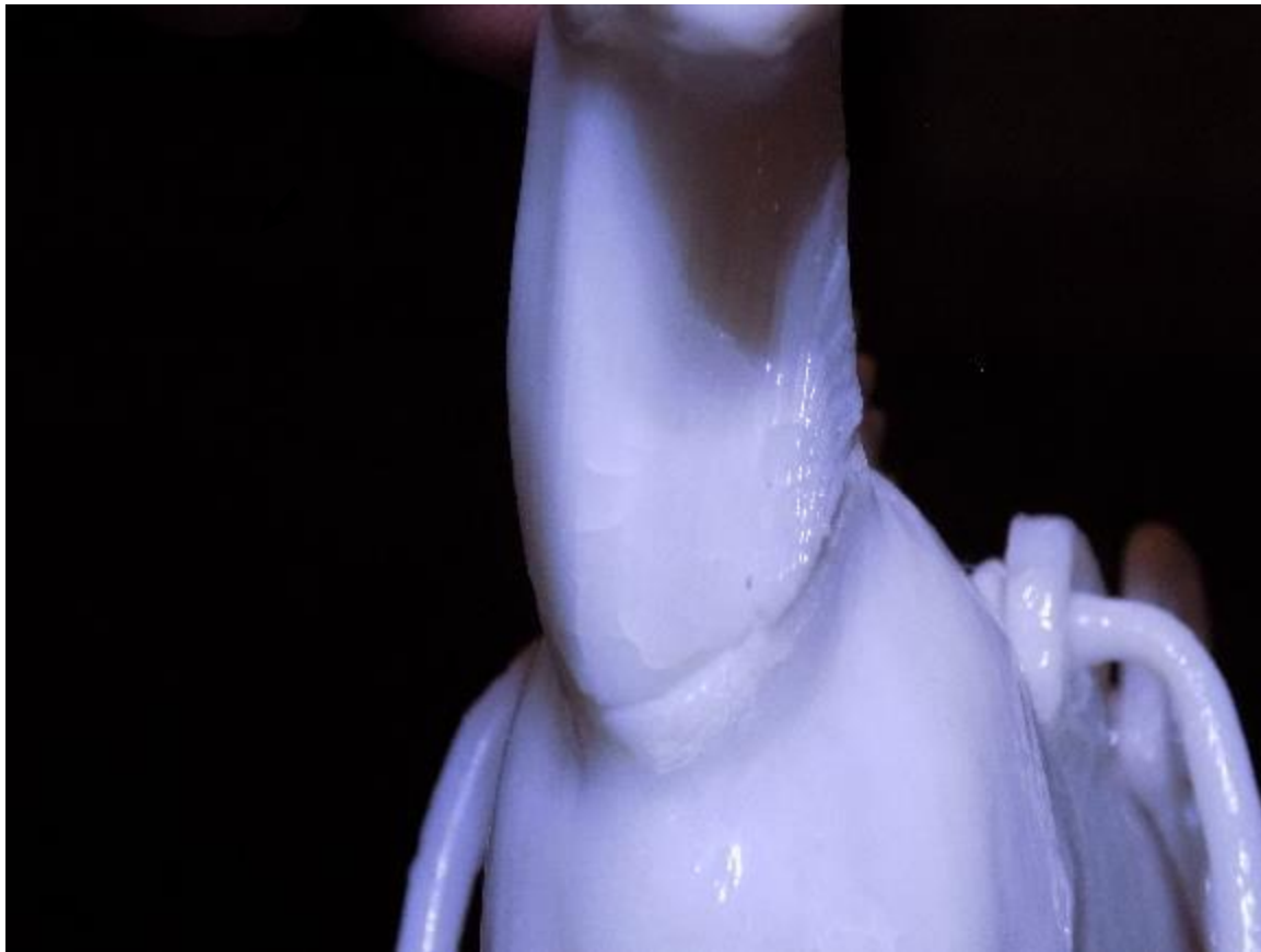
Figure 36 Cracks above seam line
