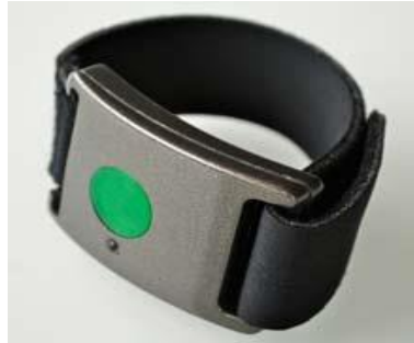
Figure 2.4 The Q Sensor measures skin conductance, temperature and motion to record a wearer's reactions to events.
