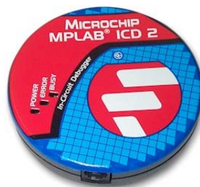
Figure 6.2 Microchip MPLAB ® ICD2 programmer
