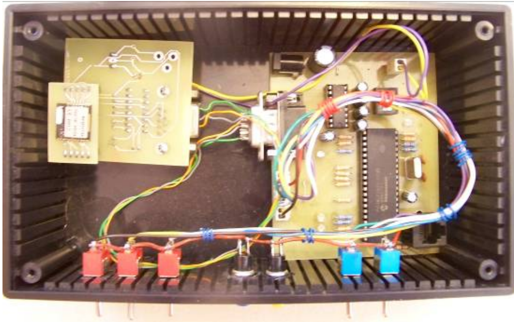
Figure 6.20 Device including controller and radio modem
