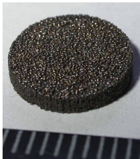
Fig. 4. Appearance of successful SLM sample. Disk with 10 mm in diameter. P = 70 \text{ W} , v = 140 \text{ mm/s} .
