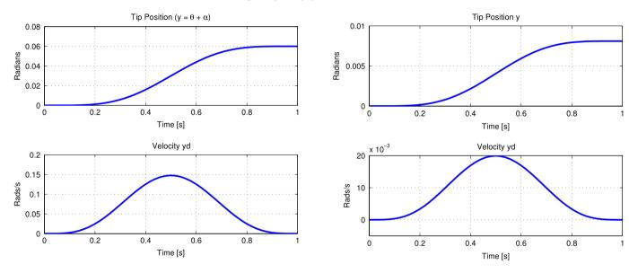
**Fig. 4.** Tip position and velocity of follower robot in open loop using Leader control input (case 1).
