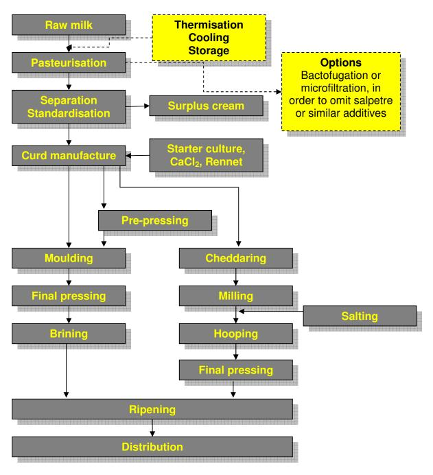
**Figure 1.** Process flow in the production of hard and semi-hard cheese (adapted from Bylund, 1995).
