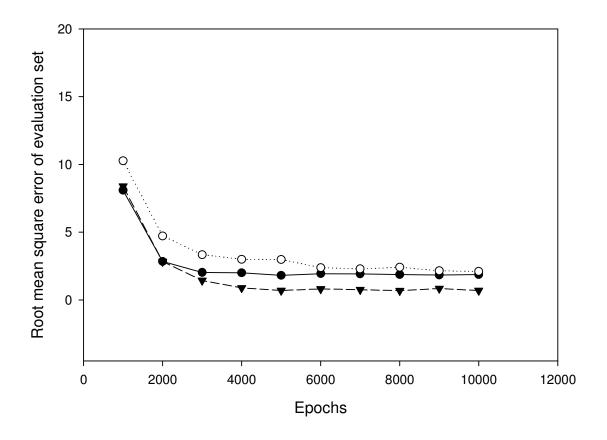
**Figure 3.** Performance of the training sets with *Lactococcus lactis* ( $\bullet$ ,  $\circ$ ,  $\blacktriangledown$  = training set 1, 2, 3). It should be noted that the recognition and prediction ability remained stable after  $1x10^4$  epochs. Satisfactory generalisation without overtraining is also noted.
