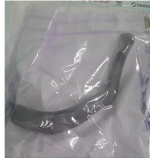
Figure 5: Customised AM jaw from Ti6Al4V powder in an EOS M280 machine
