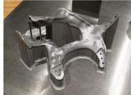
**Figure 7** - DMLS implant in Ti6Al4V
