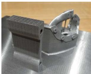
**Figure 15** - Test pieces for destructive mechanical testing
