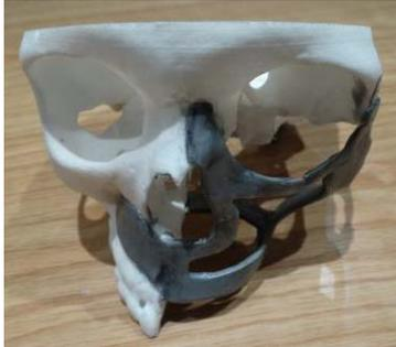
**Figure 4** - Wax model of the planned titanium frame
