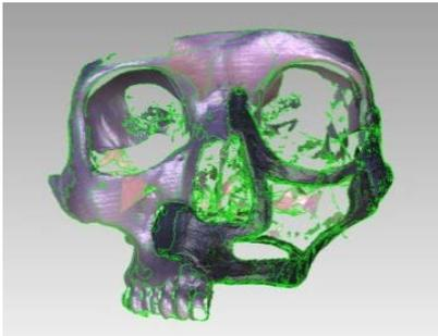
**Figure 5** - Reverse engineering data in Geomagic® software
