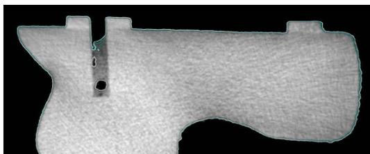
**Figure 14** - Powder trapped inside blind hole
