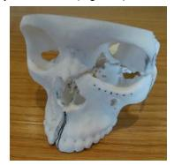
Figure 2 - Skull replica manufactured using Additive Manufacturing in PA 2200 polyamide material
