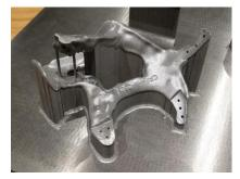
Figure 7 - DMLS implant in Ti6Al4V
