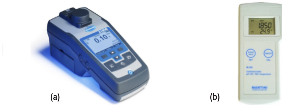
Figure 3.4 On-site measuring instruments: (a) HACH 2100Q turbidity meter; (b) MARTINI MI 806 multi probe
