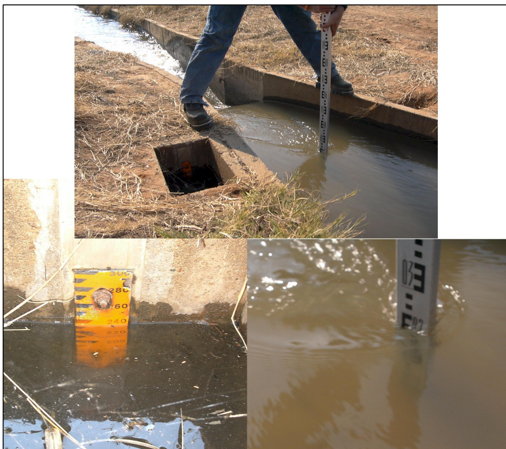
Plate 5.2: Measurements in Parshall flume in Feeder 4
