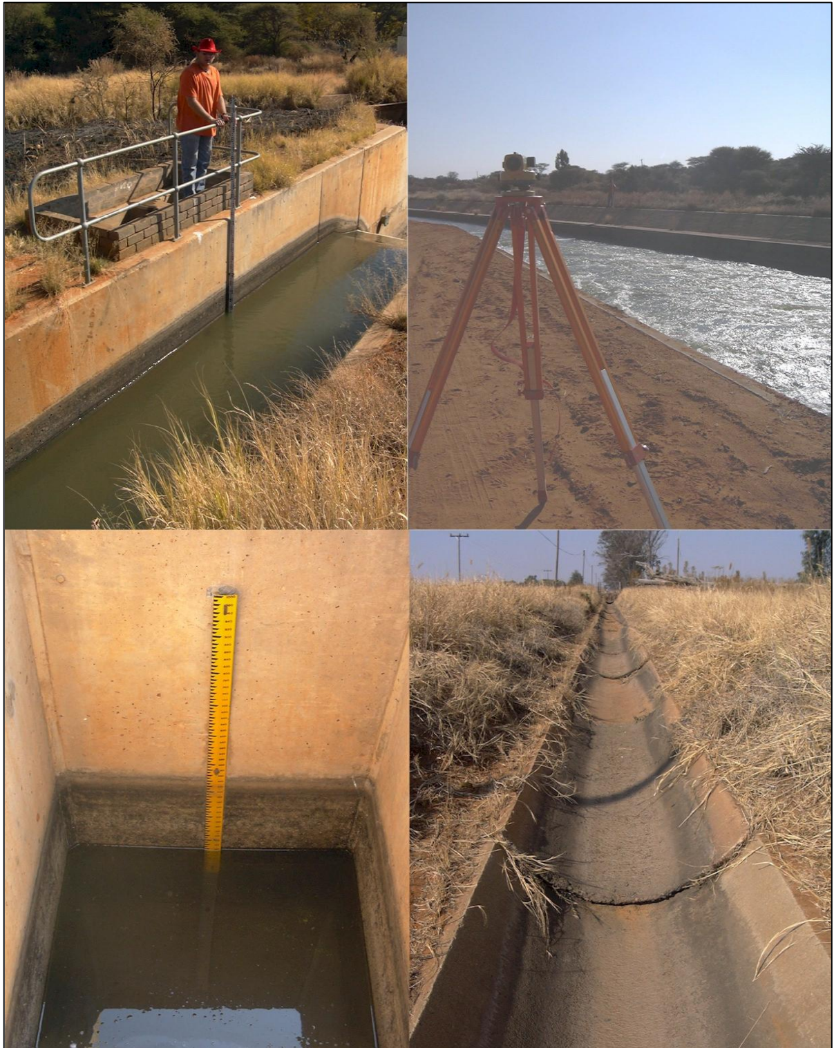
Plate 4.3: Measurements for data verification of canal geometry
